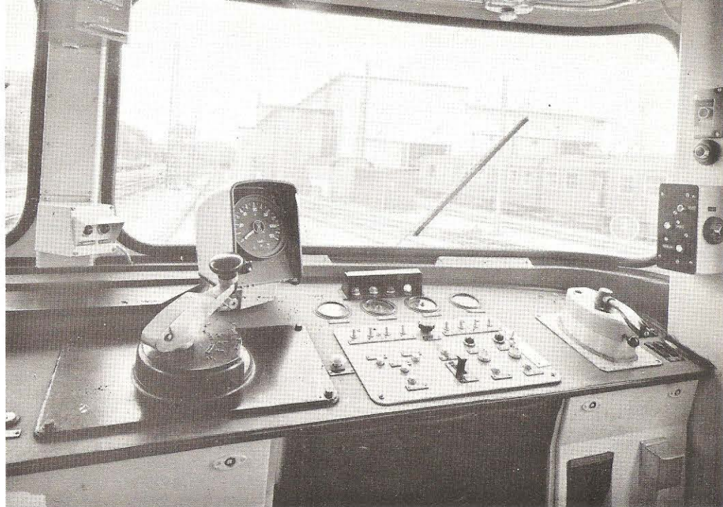
RIGHT: Driver's desk in the cab of a DSB S-Train; pushbuttons beside the door on each side permit the train to be started while the driver is looking back along the platform, thus eliminating the need for a second crew member on the train
